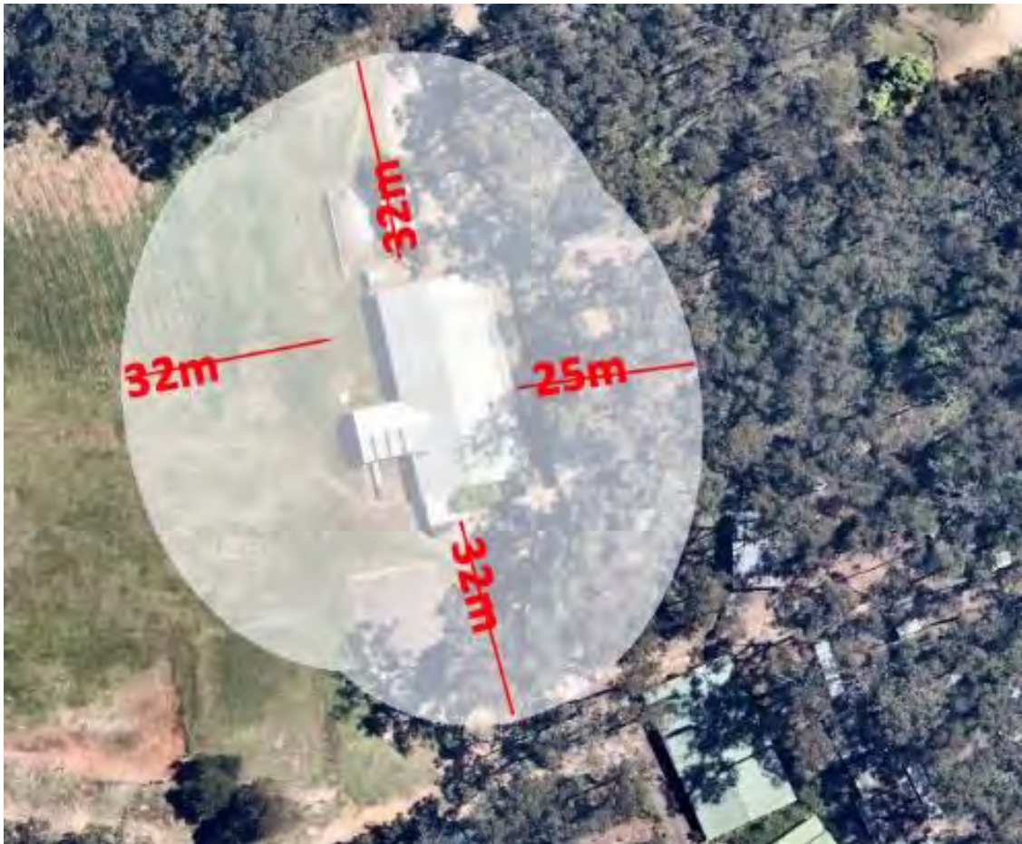
Figure 4.3. Aerial image showing the just the Inner Fuel Management Zone measured and plotted using near maps.
