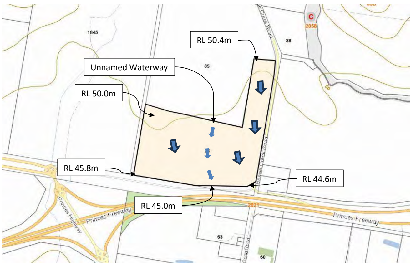
Figure 3 – Topography of the Subject Land
