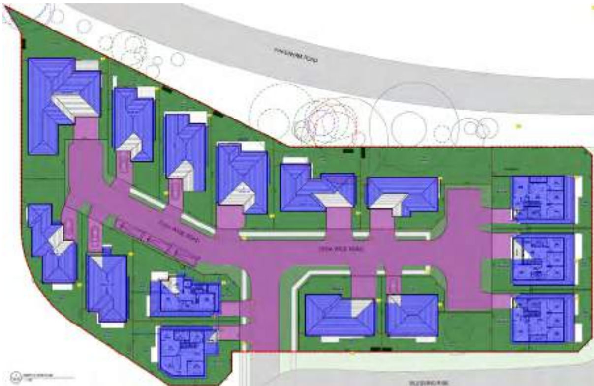
Figure 4: Roof to RWT (blue), driveway/road to raingarden (purple), and permeable landscape (green)
