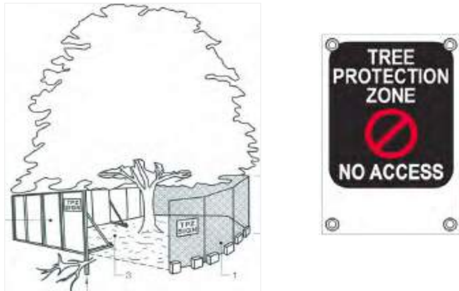
Figure 1. Above left - Example of TPZ fencing above right -Example of TPZ signage.
