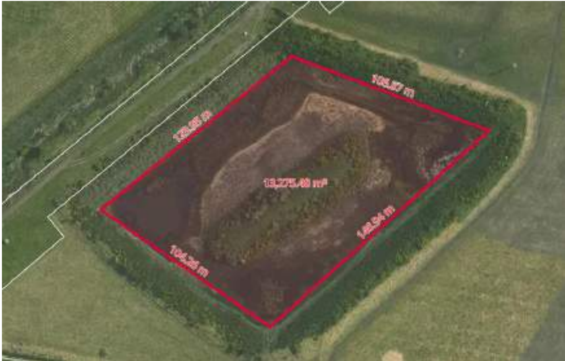
Figure 3. Dam dimensions at 500 Seven Mile Road
