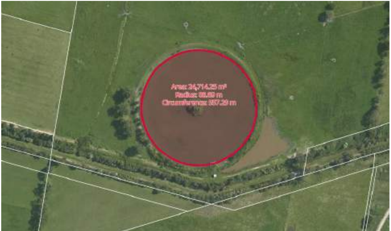
Figure 2. Dam Dimensions at 505 Five Mile Road, Pakenham
