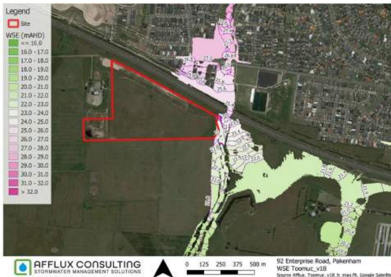
Figure 42. Preliminary Flood Levels
