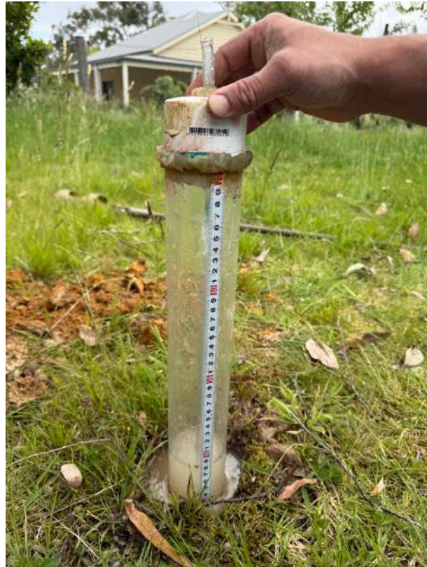
Photo 2. Soil Permeability Testing
