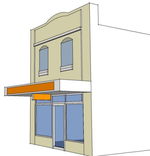
Figure 14. Verandah Fascia & Under Verandah Sign
