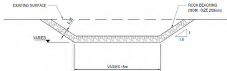
Figure 6-7 Typical section of rock-lined channel – Option 1D
