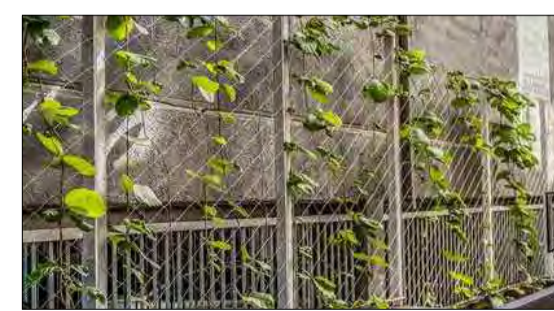
TENSILE JAKOB WEBNET 2 GREEN FACADE SYSTEM, MADE FROM STAINLESS STEEL 316 GRADE WIRE AND AVAILABLE IN WIRE DIAMETERS 1.3MM AND APERTURE OPENINGS OF 25MM-300MM THE MESH IS DYNAMIC AND STRONG. THE MESH IS MADE TO ORDER AND CAN BE ASSEMBLED INTO ANY SIZE OR SHAPE.
