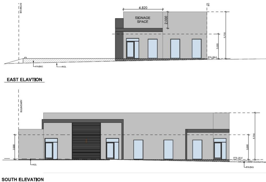
Figure 3: East and South elevation plans
