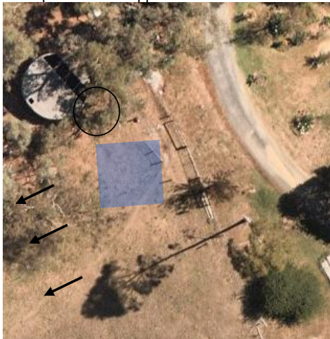
Approx. siting – no vegetation impacted – good access to the driveway Lands fall sharply approx. 10m from the back of the shed Circle for tree closest
