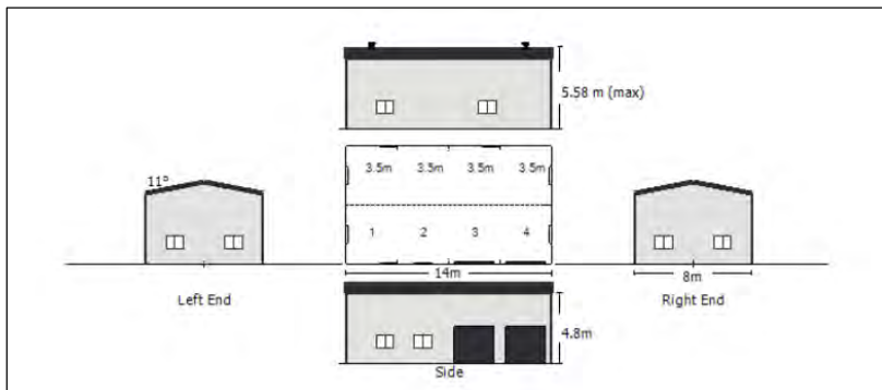
Figure 4: Outbuilding elevation drawings
