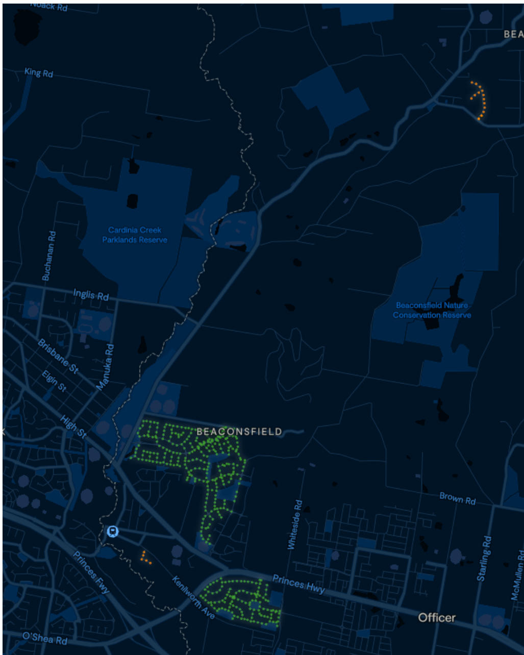
Figure A4: Mercury vapour lights intended to be replaced (green and orange) in stage 3 of mercury vapour street lighting upgrade
