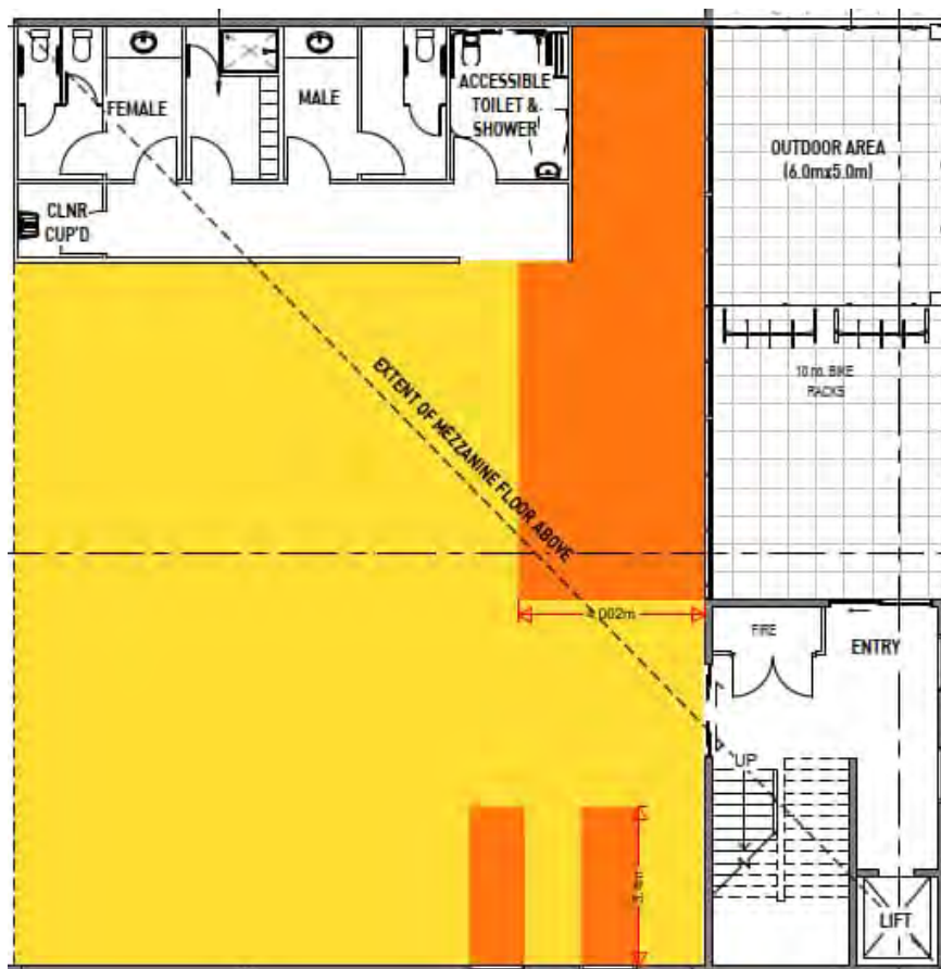
Figure 31: WH2E Under croft, compliant area marked up in orange (mark-up by SDC)
