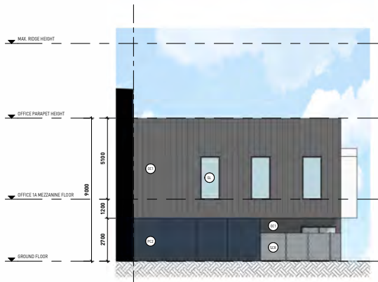
3 OFFICE 2B NORTH ELEVATION 1 : 100
