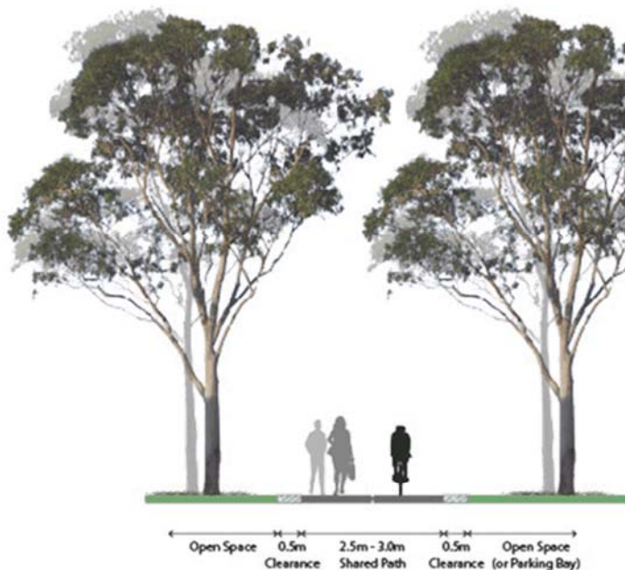
Figure 17 - Typical Shared Path cross section
