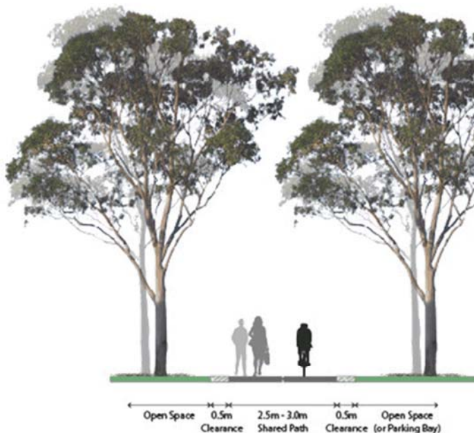
Figure 17 - Typical Shared Path cross section
